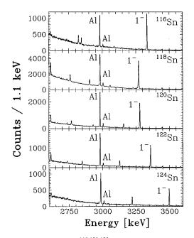
FIG. 1. NRF spectra for <sup>118,120,122</sup>Sn together with the data from our previous study on <sup>116,124</sup>Sn [17]. The peaks marked by "1<sup>-</sup>" correspond to the two-phonon excitations. Peaks labeled by "Al" stem from transitions in <sup>27</sup>Al, used for the photon flux calibration [26]. The bremsstrahlung endpoint energy in all measurements was 4.1 MeV.
