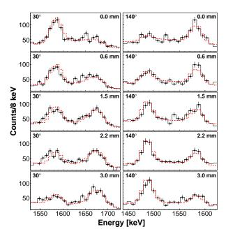
FIG. 2. (Color Online) Experimental gamma-ray spectra with statistical uncertainties (solid black) and simulated lineshapes (dashed red) generated with the best-fit lifetime  $\tau=22.4$  ps for the 1585 keV transition in <sup>18</sup>C for the 30° and 140° rings of SeGA and all five target-degrader distances. Doppler corrections were done with  $\beta_{slow}=0.2920$ .
