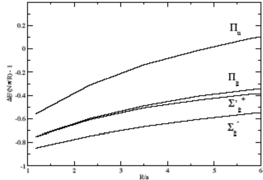
FIG. 8: Splittings between the excited energies of quasi-gluons and the ground state  $Q\bar{Q}$  energy. The values  $N$  expected from the string model are,  $N = 1$  for  $\Pi_u$ ,  $N = 2$  for  $\Pi_g$  and  $\Sigma_g'$  and  $N = 4$  for  $\Sigma_g^-$  ( $a = 0.2$  fm).
