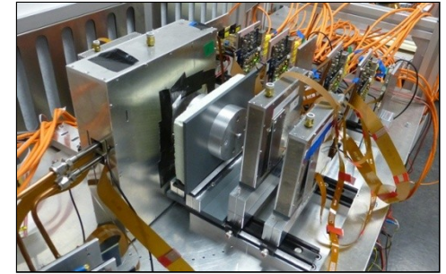
Silicon Pixel sensors MAPS for Micro Vertex detector beamtest at CERN SPS, 2012
