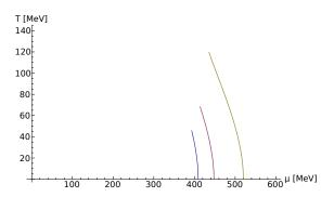
Figure X.3.: The lines show the position of the first-order phase transition between the (approximately) chirally symmetric phase (large T or  $\mu$ ) and the spontaneously broken phase (small T and  $\mu$ ) for parameter sets [C] - [E] (from left to right).
