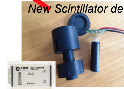
Small PMT to increase dynamic range
