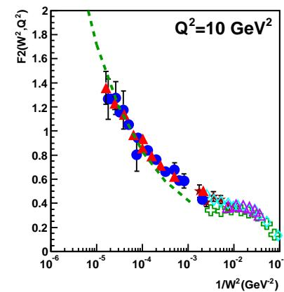
Saturation limit:  $\lim_{\substack{W^2 \rightarrow \infty \\ Q^2 \text{fixed}}} \frac{F_2(x \cong Q^2/W^2, Q^2)}{\sigma_{\gamma p}(W^2)} = \frac{Q^2}{4\pi^2 \alpha}$
