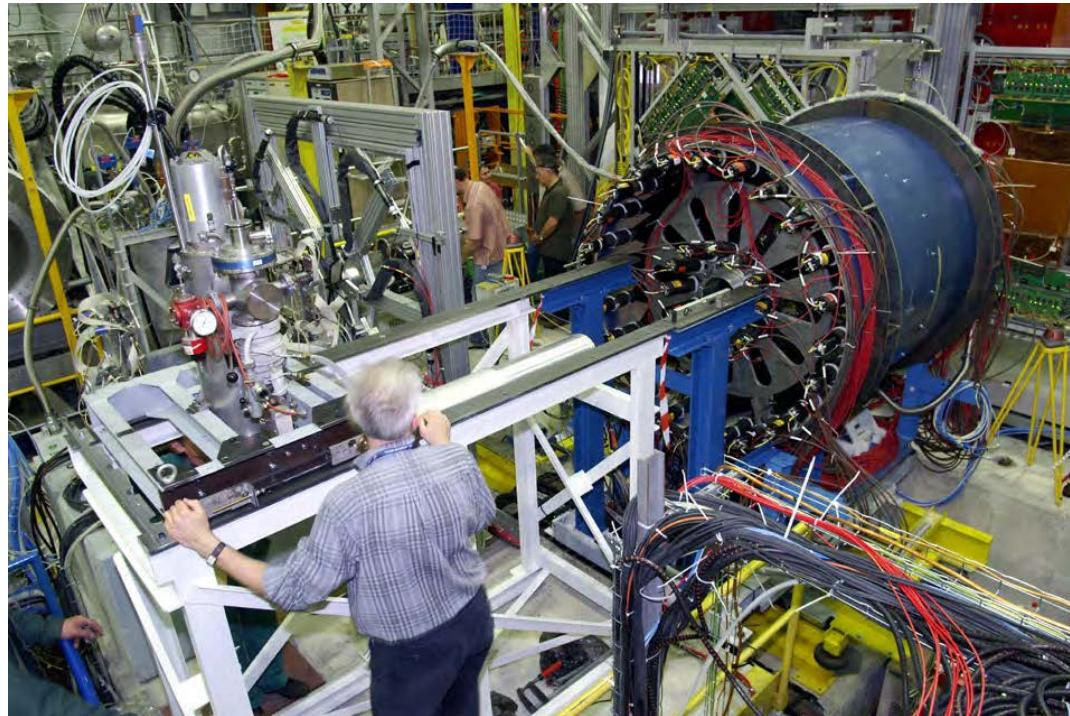
Inserting the liquid hydrogen target in the recoil detector
