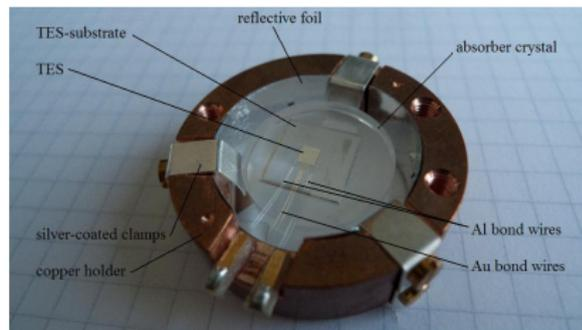
example of a realized and tested composite detector
