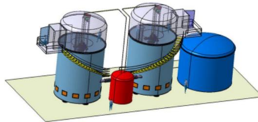
design study of the EURECA cryostat with two separate detector volumes, each stored in one water tank
