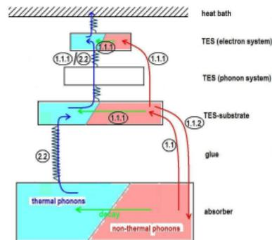
remaining *non-thermal* and *thermal* phonon propagation possibilities
