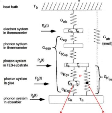
model of a composite cryogenic detector in terms of its thermal components
