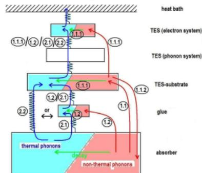
most relevant propagation possibilities for the *non-thermal* and *thermal* phonons
