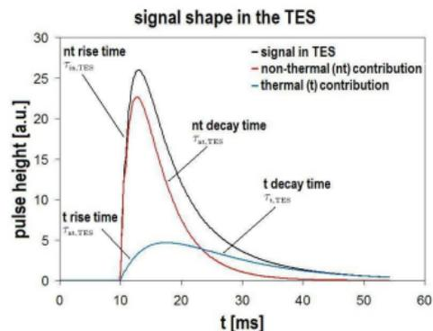
*signal shape in the TES of a cryogenic detector with the TES directly deposited on the surface*
