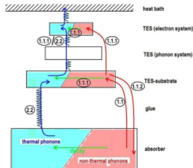
remaining *non-thermal* and *thermal* phonon propagation possibilities
