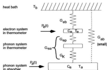
*model of a cryogenic detector with the TES directly deposited on the surface in terms of its thermal components*
